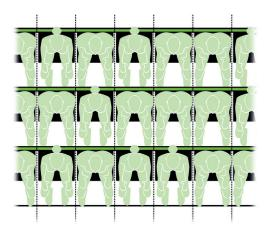
If, when standing, spectators cannot make the necessary adjustments, those at each end of the seating row will inevitably encroach onto the radial gangways, as shown below. This runs contrary to one of the basic principles of safety management at sports grounds and other places of public assembly; that all radial and lateral gangways be kept clear at all times during an event (see Section 8.7 of the *Green Guide*).
