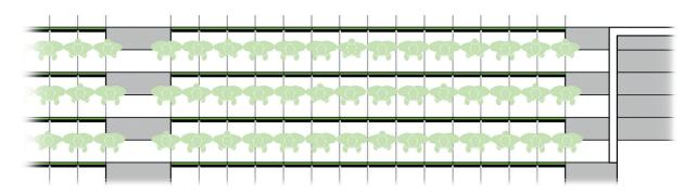
If, however, spectators are able to make the necessary adjustments, and there is no encroachment onto radial gangways, as seen below, management will still need to demonstrate that the space per spectator is not less than the recommended minimum for standing spectators in a seated area of 0.20m<sup>2</sup> per person (see Section SG01 2.3.f).
