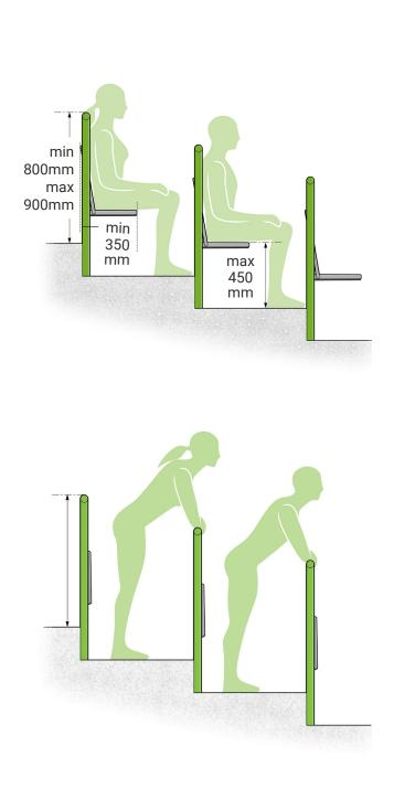
Barriers incorporated into seats, as described in Section 12.21 of the *Green Guide* and **Section SG01 2.3.d**, should be designed to a minimum height of 800mm and a preferred height of 900mm, measured from the datum, and should resist safely a minimum horizontal imposed load of 2.0 kN/m length.
